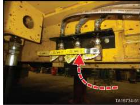
Close the valve under the hydraulic reservoir
