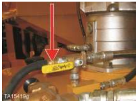
Close the hydraulic reservoir air valve
