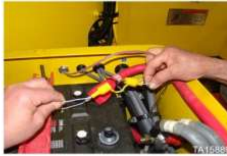
Fire suppression in-line fuse located in loader battery box on some machines
