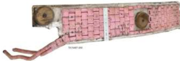
Typical ceramic heater, recorder and elements
