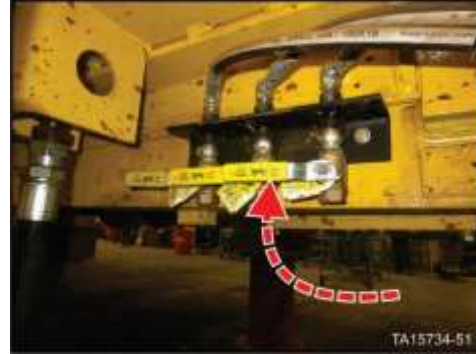
Close the valve under the hydraulic reservoir
