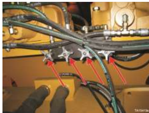
Close hydraulic bleed valves in front frame
