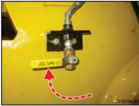
Close the valve under the hydraulic reservoir
