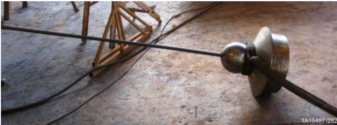
Install the alignment bar and hoist strap
