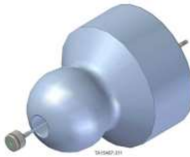
Ball plug – grease through ball
