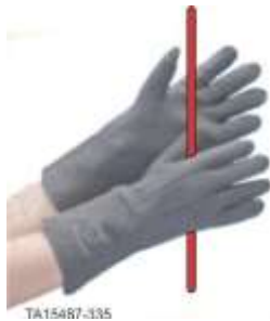
Check to make sure gauge rod freely enters all locations
