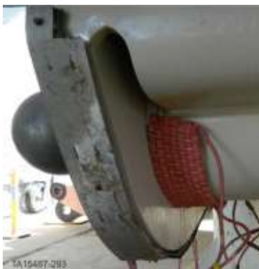
Typical ceramic heater locations on inside of frame
