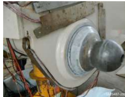
Typical ceramic heater locations on outside of frame
