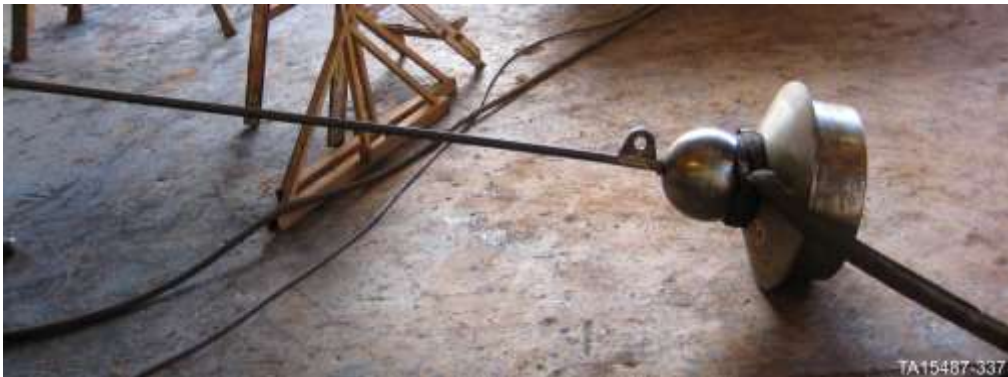
Install the alignment tool and hoist strap
