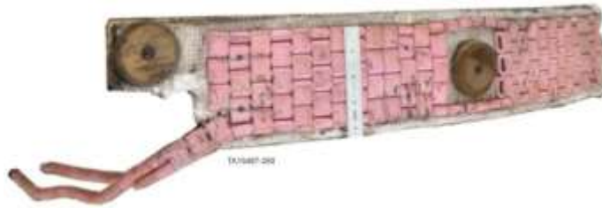
Typical ceramic heater, recorder and elements
