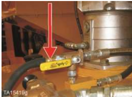
Close the hydraulic reservoir air valve
