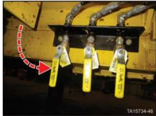
Figure 3. Open air reservoir bleed valves
