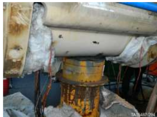
Typical ceramic heater locations on inside of frame
