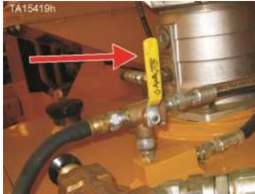
Hydraulic reservoir air valve handle UP
