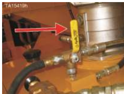
Hydraulic reservoir air valve handle UP
