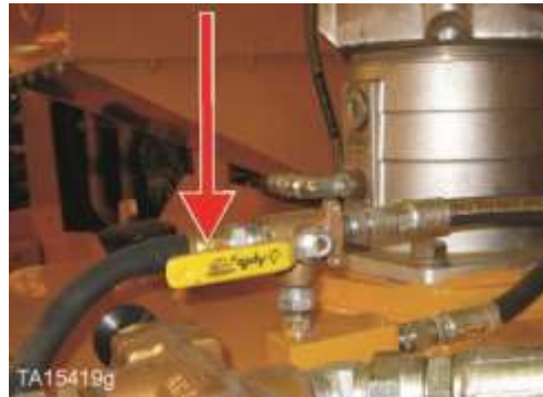
Close the hydraulic reservoir air valve
