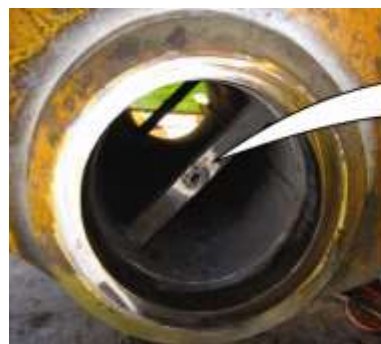
Install nut in middle of cross support
