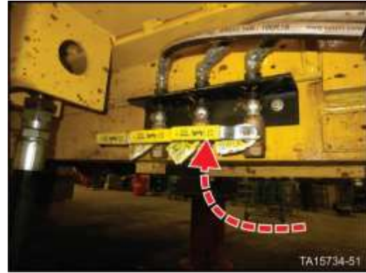
Close the valve under the hydraulic reservoir
