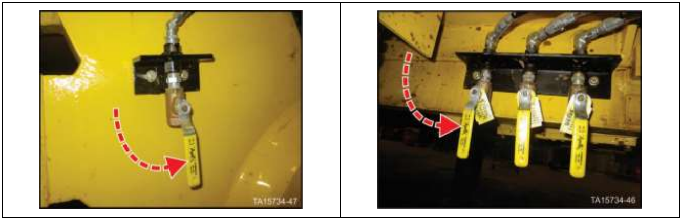
Figure 2. Open air reservoir bleed valves
