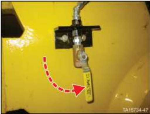
Figure 3. Open air reservoir bleed valves
