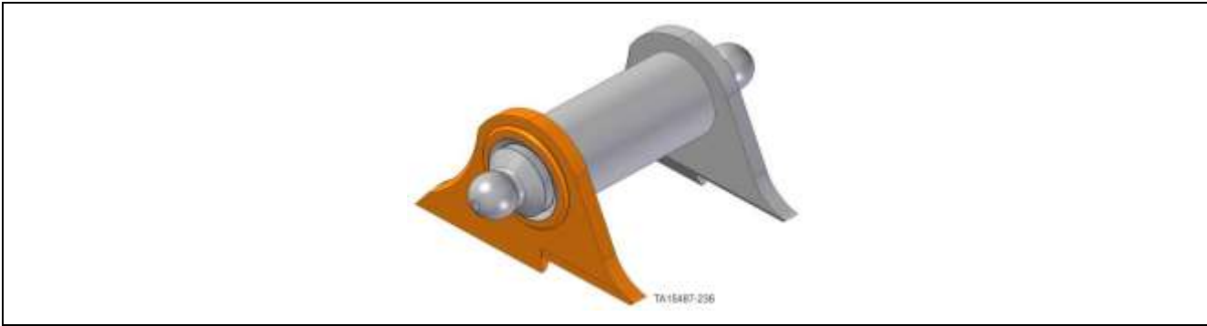
Sub structure assembly with hot slab in place
